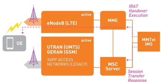
With acknowledgements that the commands have been executed, the user's device and the IMS/MMTel—still in control of the user's voice call in progress—switch to the CS network to continue the call. (Figure 8)
