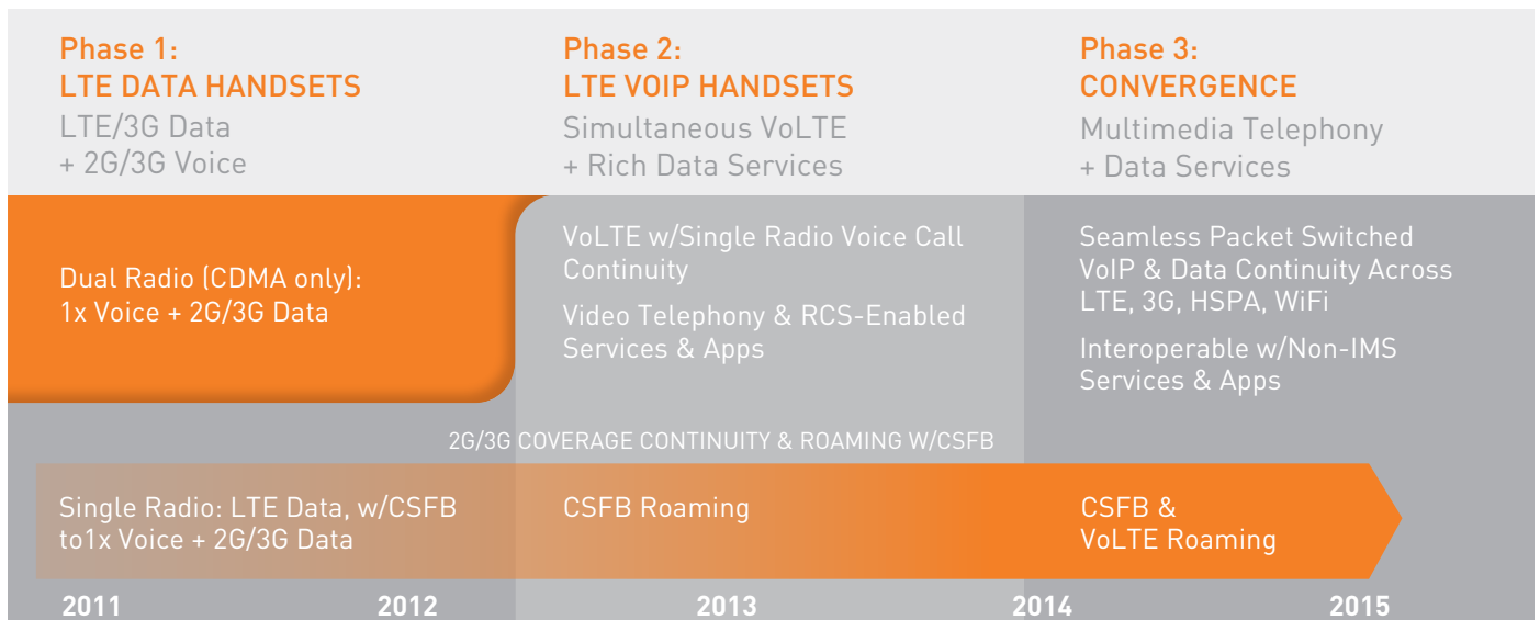
Figure 2 The 3 phases of LTE voice evolution.
