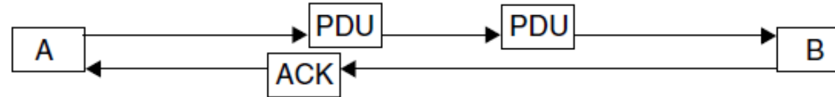
Type 2 connection-oriented service
